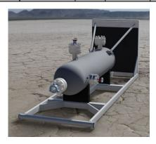
Cyclonic Sand Traps: This style utilizes the intake of hydrocarbons and solids at high velocity accompanied by the momentum of the cyclone action to separate out sand through internals, keeping more sand away from testing equipment.
